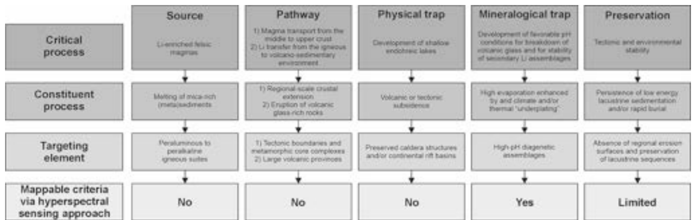
Fig. 15. Mineral system approach (MSA) applied to volcano-sedimentary Li deposits, with reference to the potential of hyperspectral sensing to target mappable criteria related to the development and preservation of suitable mineralogical traps (see section 6.3 for details).
