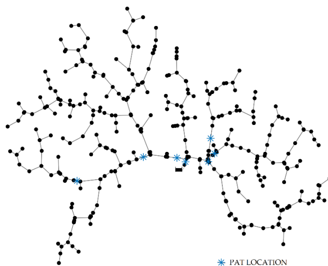
Figure 3. PAT location within the case study network according to the global optimum solution.
