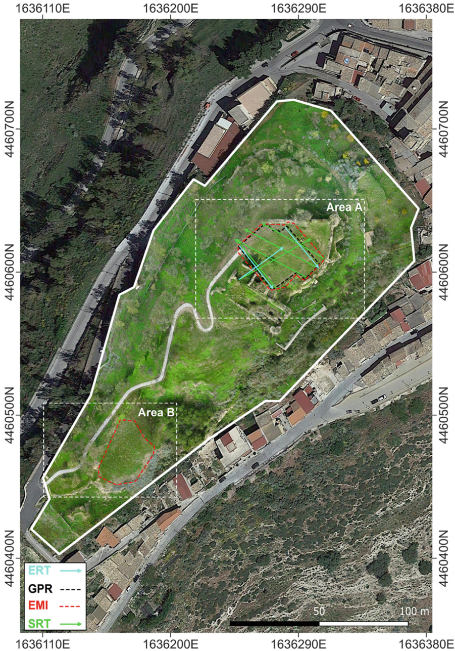
Fig. 4. RGB image obtained through aerial photogrammetric survey with indication of the geophysical survey.
