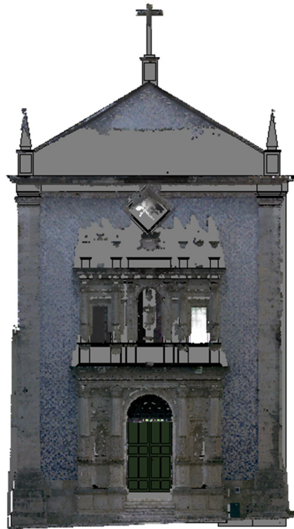
Figure 4. Point cloud on the 3D model in Revit.
