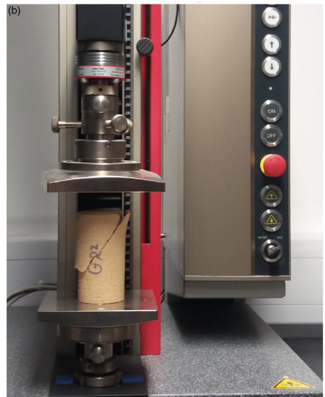
Fig. 5. (Colour online) Mechanical testers used in this study: (a) ring-shear tester sketch (modified after Schulze, 1994) and (b) uniaxial compression tester.
