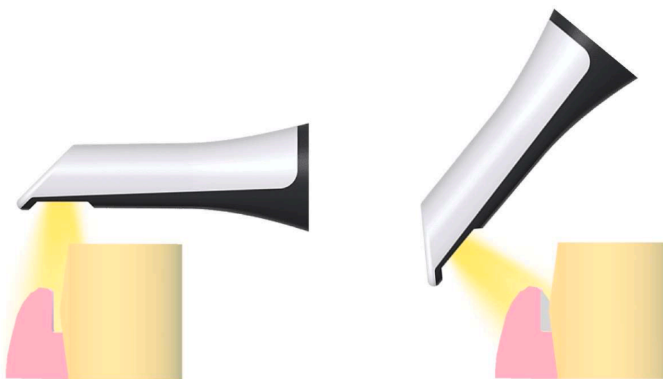
Fig. 10. Representative schematizations of different angulations of the IOS light beam on vertical preparations. Different angles of the light beam and possible anatomical undercuts are related to the presence or absence of shadow cones.
