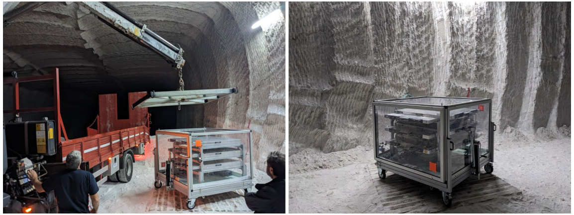
Fig. 10. Images show the deployment and the positioning of the MURAY detector inside the Realmonte salt mine. Researchers assist with the operation, highlighting the scale and logistical complexity of deploying a ton of instrumentation in such a unique underground context.
