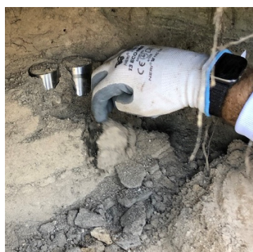
Figure 3. Example of manual undisturbed sampling.
