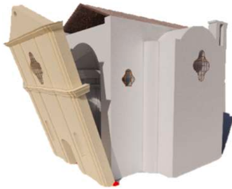
Fig. 8. Example of façade overturning characterized by the formation of a cylindrical hinge at the base of the masonry wall. The case shown refers to the Church of the Addolorata, one of the buildings included in the dataset.
