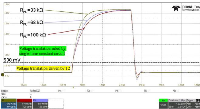
Fig. 6: Output waveforms of the TI LSF0102 level shifter for different values of the pull-up resistor.
