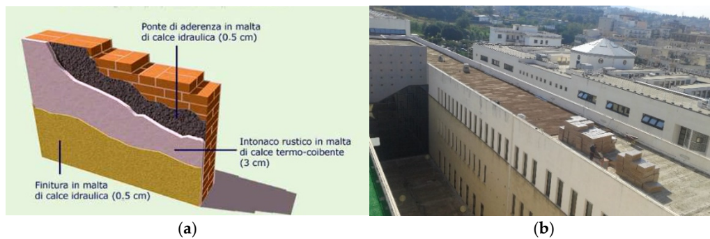
Figure 2. (a) Multilayer external insulating super plaster named “volcalite”. Source: Authors. (b) Real-world ecological retrofitting of buildings at Mediterranean University of Reggio Calabria (Italy), Department of Architecture. Flat roof/terrace “passivation”/insulation with insulating/ventilated bio natural cork panel named “genius”. Covered by insulating “vermiculite screed”, waterproof bituminous membrane and ventilated raised adjustable floor tiles. Source: Authors.
