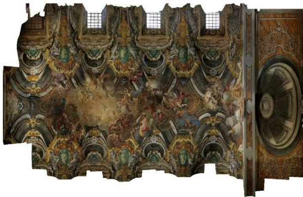
Figure 9. Cylindrical projection of the geometry of the vault and the paintings that decorate it
