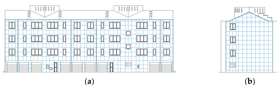
Figure 6. Schematic configuration of the reinforcement: longitudinal (a) and transversal (b) façades of the retrofitted building.
