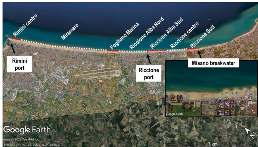
Fig. 15. Stretch of coast between Rimini and the last detached breakwater of Misano Adriatica, the red/white dotted lines indicate the sub segments for which the volumetric analysis by Arpae has been carried out.
