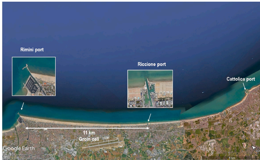
Fig. 12. The sand beach compartment between Rimini port and Riccione port, included in the wider physiographic unit of Rimini-Cattolica. The smallest panels give an insight on the port's jetties.
