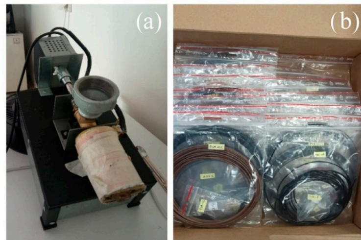
Figure 1. (a) Single screw extruder: It consists of a hopper, a main motor rotating a single screw, and a heated nozzle producing filaments of 1.75 mm diameter. (b) Custom-made and commercial filaments.
