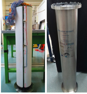
Fig. 3. Left: the detector without the steel cylindrical shell. Right: the detector assembled into the shell.
