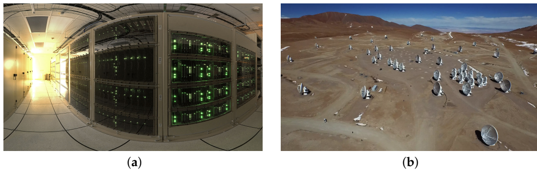
Figure 1. (a) The ALMA correlator in the ALMA array operation site (AOS) technical building is composed of four identical quadrants with over 134 \times 10^6 processors, performing up to 17 \times 10^{24} operations/s (Image credit: ESO). (b) A panoramic view of the ALMA array, located at an elevation of 5000 m on the Chajnantor Plateau in the Chilean Andes. The AOS is the small building left of picture center. The tight clump of antennas near the image center is the ACA (Image credit: JAO).
