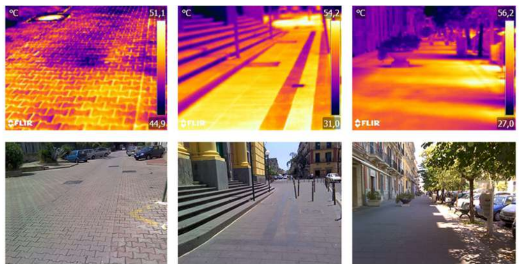
Figure A5. Thermographic surveys of the 3 July 2015 of "Lotto PSER" in Fratelli Grimm Avenue (P19), Vincenzo Aprea Square (P29), Margherita Avenue (P31).
