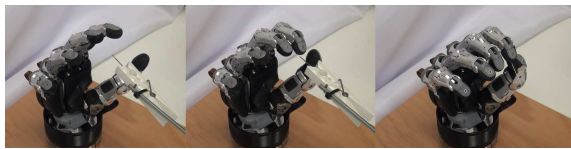
Fig. 7. Precision grasp example of a very small object: needle.
