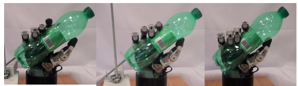
Fig. 9. Power grasp example using the full-DoF search space: bottle.
