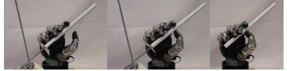
Fig. 5. Precision grasp with five fingers example: small cylinder.
